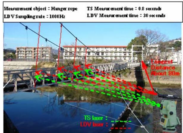
Figure 7. Automated remote measurement system using LDV and Total Station.
