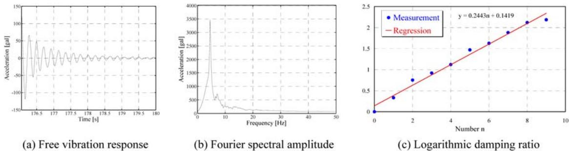
Figure 13. Simple modal testing using wireless accelerometer.
