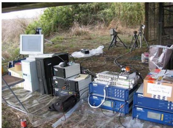
Figure 1. Equipments of measurement using LDVs.
