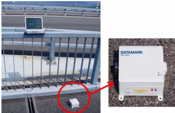
Figure 9. Wireless tri-axial MEMS based accelerometer.
