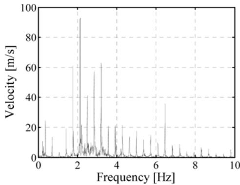
Figure 4. Example of Fourier spectral amplitude of a cable.
