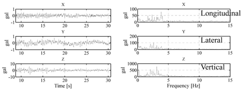
Figure 12. Measurement results by a wireless LAN accelerometer.
