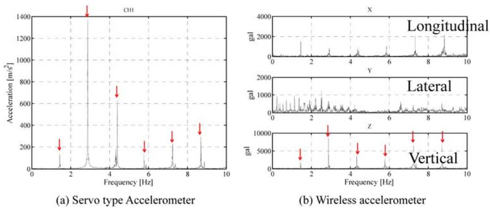
Figure 11. Comparison of Fourier spectral amplitudes (Arrows indicate natural frequencies).
