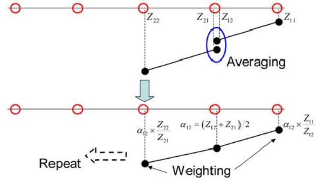
Figure 16. Connection of partial mode shape.
