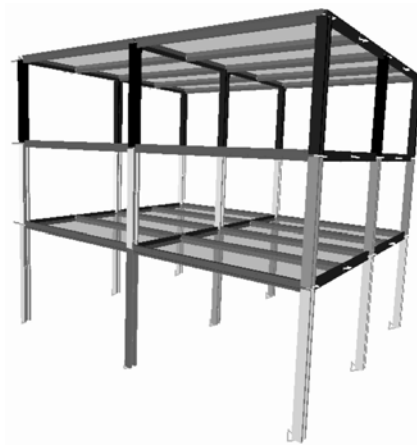
Figure 6. The 3-storey non-sway frame under floor loads.
